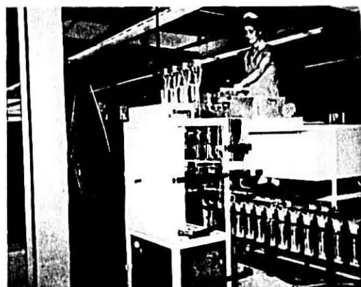
Weigher fills buckets with correct amount of spaghetti. Buckets automatically dump into form over bottom-sealed carton filling the carton. Conveyor carries weighed package to top sealer and compression unit.
